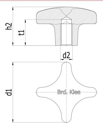
$\begin{array}{lll} d1 & = 40 \\ d2 & = M8 \\ h2 & = 25 \\ h4 & = 13 \\ t1 & = 15 \\ Weight in (g) = 62 \end{array}$
